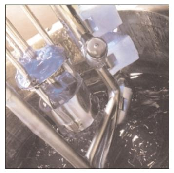
AN INTEGRATED SYSTEM WITH THREE SEPARATE MIXERS FOR VARIABLE-SHEAR BATCH PROCESSING AND A COMPUTER INTERFACE FOR INSTANT ANALYSIS
