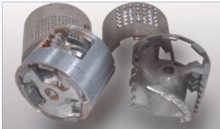
Toothed impeller/liner combination showing full open discharge, 1/4" grid and 1/16" grid.
