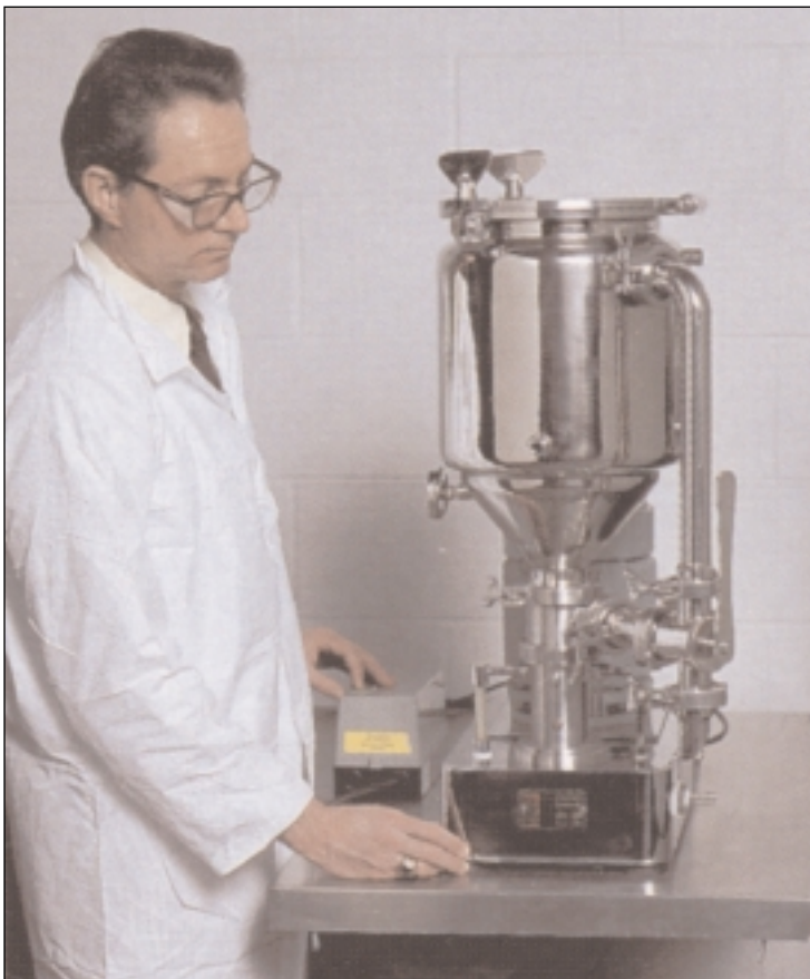
Model 2x1 Dicon unit with 12 liter jacketed mixing vessel and recirculation piping and 3-way valve.
